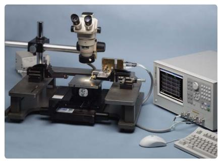
Figure 16. Agilent E4991A with probe station
