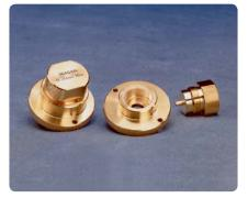
Figure 15. 16454A Magnetic material fixture
