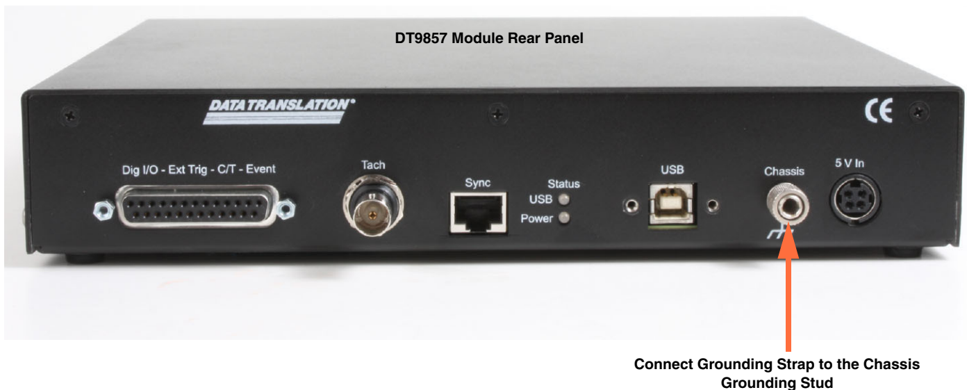
Figure 6: Connect a Grounding Strap to the Grounding Stud on the DT9857 Module
