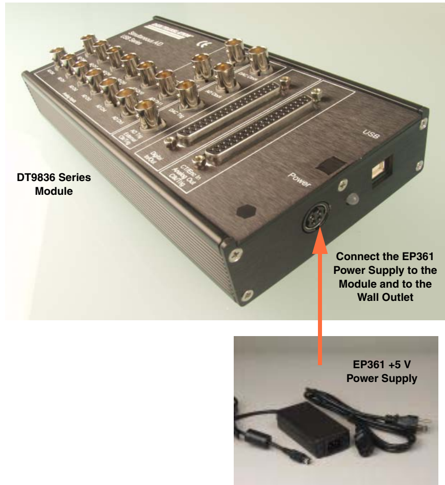
Figure 3: Attaching a +5 V Power Supply to the DT9836 Series Module
