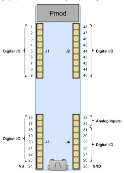
Figure 7.1 DIP Pin Diagram
