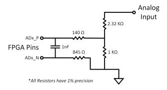
Figure 7.2.1 Analog Input Circuit
