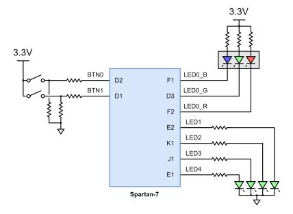
Figure 6.1 Cmod S7 Basic I/O
