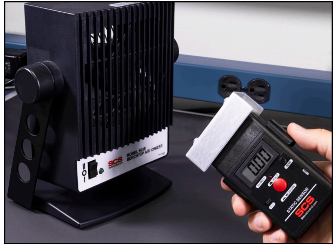
Figure 9. Using the Static Sensor with Conductive Plate to measure the offset voltage of a benchtop ionizer
