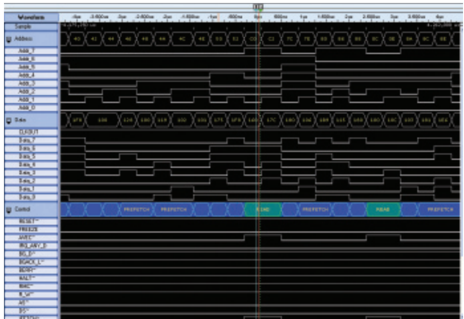
Figure 1. Logic Analyzer acquisition of a microcontroller's clock, address bus, data bus and control lines.
