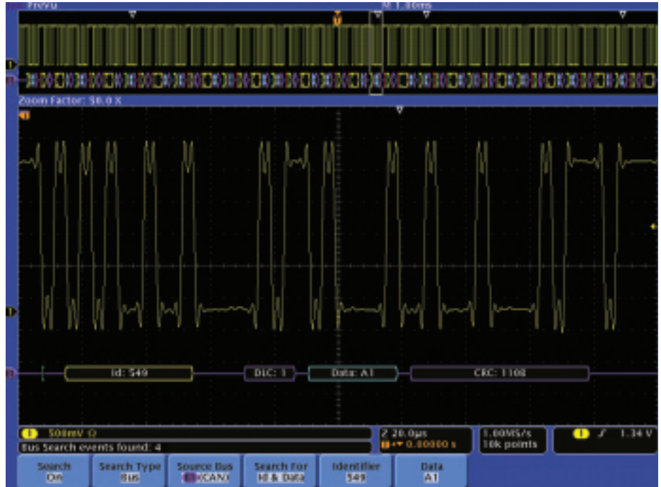
Figure 28. Searching on specified identifier and Data in a CAN bus acquisition.
