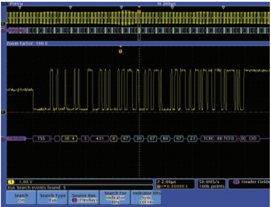
Figure 26. Triggering on Frame ID and Cycle Count, Searching through acquired data for Startup Frames.
