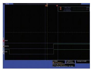
Figure 22. MSO triggering on the D-Flip-Flop data changing in the setup/hold window between cursor 'a' and 'b' around the rising clock edge.
