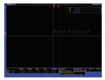
Figure 9. TTL Burst Signal.
