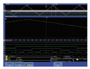
Figure 28. Correct operation with one 3F hex value at each ramp peak.
