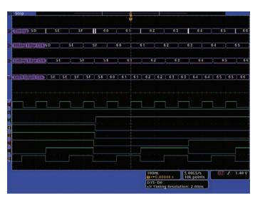
Figure 2. Example of a timing acquisition on the MSO Series. Four parallel buses have been defined and decoded using the device's clock signal.
