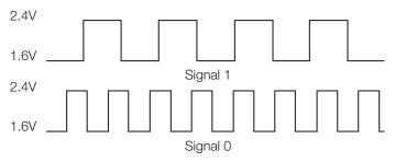
Figure 12. LVPECL signal zero with 50 ns period and signal one with 90 ns period.
