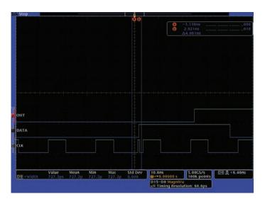
Figure 17. MSO capturing a 727.3 ps clock glitch.
