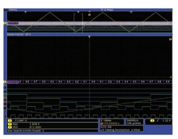
Figure 29. Correct operation with one 00 hex value at each ramp valley.
