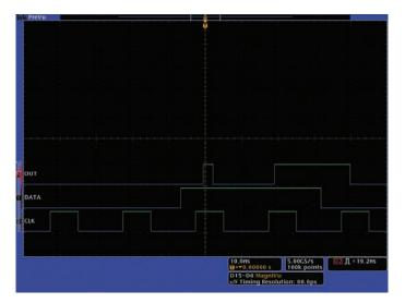
Figure 19. D-Flip-Flop Q output error.
