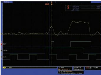
Figure 20. D-Flip-Flop Q output error with analog insight.
