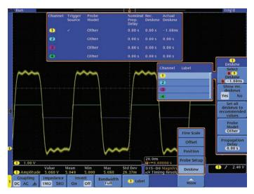
Figure 7. Analog channel time aligned with the digital channel.
