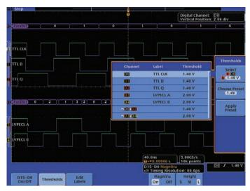
**Figure 1.** Mixed logic families (TTL & LVPECL) threshold settings on the same MSO4000 digital probe pod. The top three channels are TTL signals with a threshold of 1.40 V and the bottom two channels are LVPECL signals with a threshold of 2.00 V
