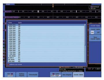
Figure 3. Decoded data is shown in an event table which is similar to a logic analyzer's state acquisition display.
