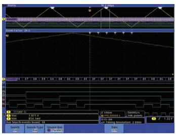
Figure 27. Wave Inspector navigation jumps to marks at 3F hex values at test signal
