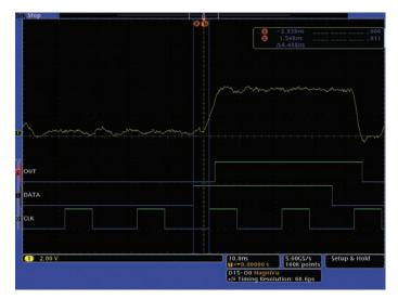
Figure 21. D-Flip-Flop Q output correctly working with 4.488 ns setup time before the risina clock edae.
