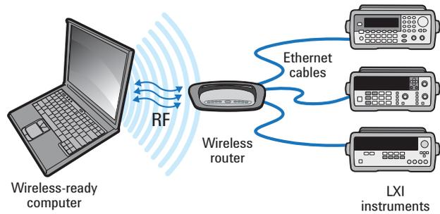
**FIGURE 1. Wireless-ready computer with single wireless router**
