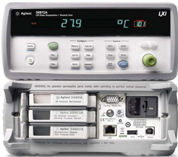
FIGURE 5. Agilent 34972A LXI data acquisition/switch unit.
