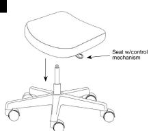
Place seat with control mechanism onto the end of the pneumatic cylinder. Sit on seat to secure fit onto cylinder.
