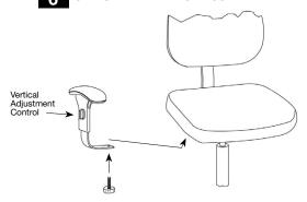
Slide arm bracket into mounting plate attached underneath seat. Tighten handwheel securely.
