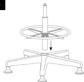
Slide the cylinder into the center of the base.
