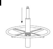
Slide footring (if enclosed) onto cylinder. Ensure the tubular ring faces upward. Tighten handwheel securely.
