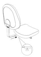
Slide the back support bar into channel of control mechanism attached underneath the seat. Tighten handwheel securely.
