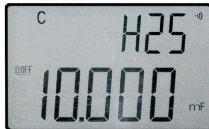
Compare mode in the U1701B reduces test set-up time for capacitor sorting.
