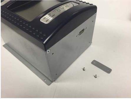
Connect the RFT Transmitter to the X-PAQ controller with the supplied 9-pin cable.
