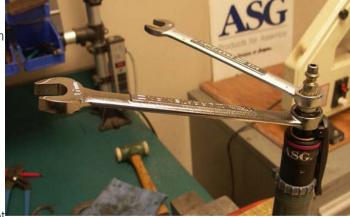
If the air inlet is removed from inline lever start tools the cone spring and ball can fall out. Missing parts are not covered under warranty.
