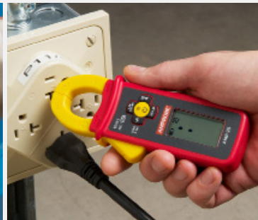
The non-contact voltage (NCV) function checks for voltage presence.
