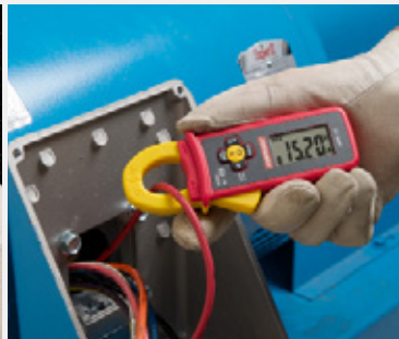
Utilize the inrush current function for motor start-up monitoring.
