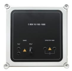
The C-Box 10/100-1000 is used to bypass the power source during ripple testing. It comes in a compact box containing two capacitances of 10 and 100 uF. The value can be selected by setting the jumper on the front panel of the box.
