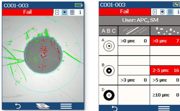
**Pass/Fail results in seconds:** With the press of a single button, FOCIS Flex auto-focuses, captures and centers the end-face image, applies Pass/Fail rules, displays image and Pass/Fail results. Captured Pass/Fail results are easily viewed in either Image or Table view.
