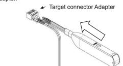
3. Push the Outer Shell to start cleaning the target connector end face. An audible "click" sound indicates end of cleaning process. Close the cover after use.
