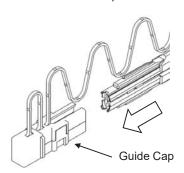
2. Insert tip of cleaner into the target connector Adapter.
