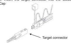
3. Push the Outer Shell to initiate the cleaning the target connector end face. An audible "click" sound indicates end of cleaning process. Close the cover after use.
