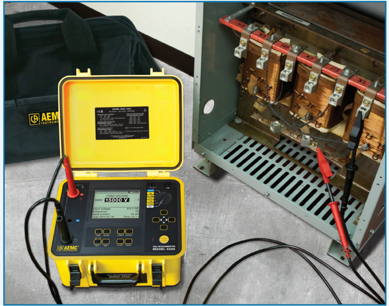
Model 6555 performing an insulation test.
