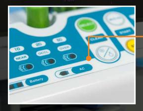
Bond printed polycarbonate to polyester in a membrane switch with 3M™ Membrane Switch Spacer 7956MP
