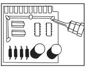
Quick, convenient, low-cost method to fasten rework wires, jumper wires, etc., at corners and along lengths to help prevent movement. Jumper wires are added to redirect circuits or repair a printed circuit board. Secure attachment of jumper wires helps improve the appearance and quality of the repaired PCB.
