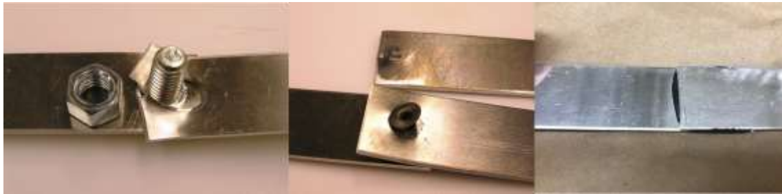
Figure 6. Failure of T6061 aluminum (0.063" thick) bolted together and the rivets upon tensile force application vs. adhesively-bonded aluminum.
