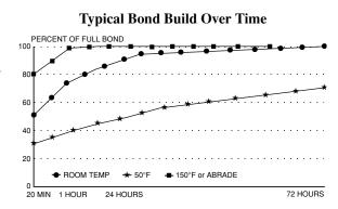
strength can be achieved more quickly by exposure of the bond to elevated temperatures (e.g. 150°F [66°C] for 1 hour).
