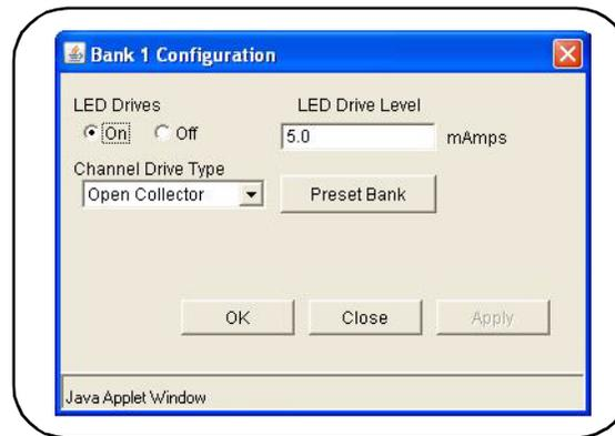
Figure 4-5. The Bank (Distribution Board) Configuration Window.
