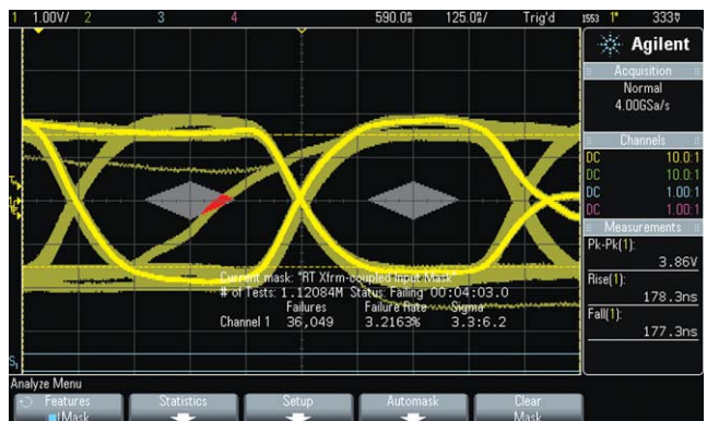
Figure 7: MIL-STD 1553 BC to RT xfrm-coupled input mask test reveals a shifted bit that violates the pass/fail mask.
