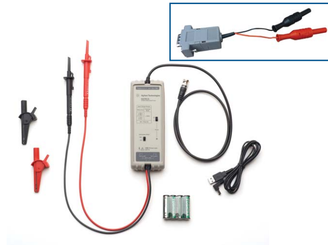
Figure 9: Agilent N2791A 25-MHz differential active probe.
