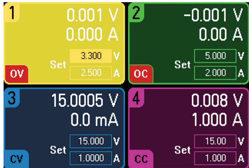
Figure 8: Power supply front panel showing over-voltage protection, over-current protection, constant voltage, and constant current mode
