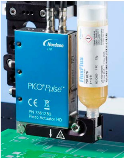
PICO Pulse® jetting FluxPlus onto a PCB.
