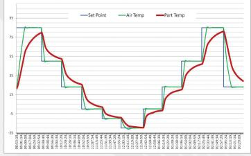
DUT never quite reaches the temperature setting. Longer test time if you actually wait for the DUT to reach Set Point.
