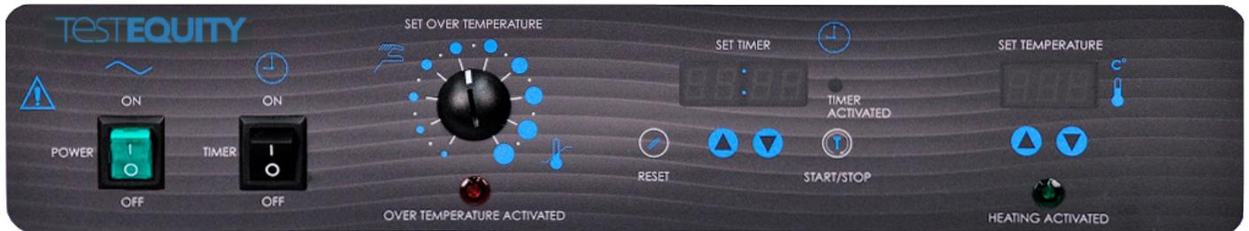
Figure 9: FOV2 Control Panel
