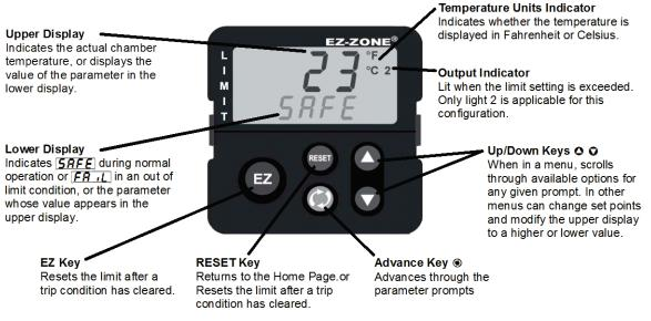
Figure 5.1 – Limit Controller Keys and Displays
