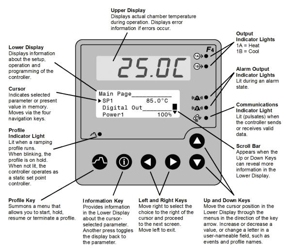
Figure 4.1 – F4 Controller Keys and Displays
