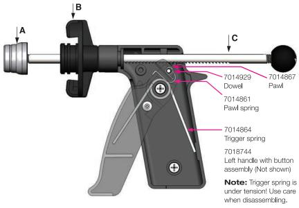
**Important:** Trigger must be in **R** position during disassembly and assembly.
