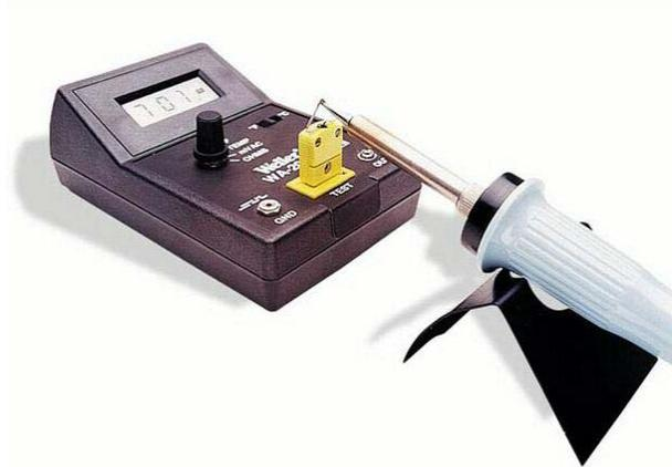
NOTE: Actual temperature readings using the pyrometer method will most likely be greater than 30 to 60 degrees F lower than the soldering tip is actually operating at. Even though it is not intended to be an accurate form of measurement, the level of accuracy or how low it may read when measuring the temperature with a contact device is still based on many factors, such as the cleanliness of the tip, operator pressure, amount of solder on the tip, angle of contact, etc.
