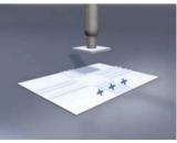
observed cases for example, where the chips were placed onto charged bare printed circuit boards (PCB's). The PCB's were initially charged from the processing operations leading up to their contact with the chip. Printed circuit wiring can discharge into the chip in this case...which is a "mini" machine model (MM) failure mode.
