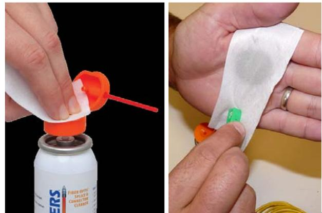
As shown in the photos, above, one small spot on the wipe should be dampened with the fast-drying fluid. Just flip open the dispenser as shown and press down to dampen the wipe. Then place the end-face on the damp spot and drag it across the wipe to a dry area. After lifting the connector from the wipe, the connector will be dry and static-free.
