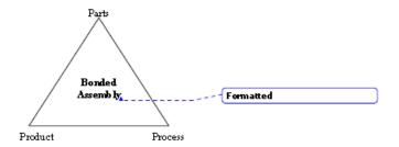
To select an appropriate adhesive for an application, a designer should consider how the device will be assembled, and what substrates will be bonded. It is also critical that the adhesive specified during the design phase is appropriate for the production process.
