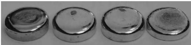
Figure 1. Comparative solder button showing different surface finishes.
