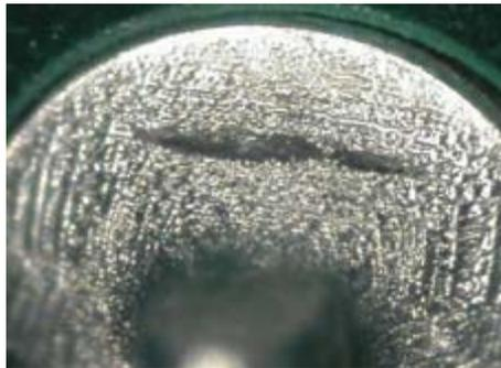
Figure 2. SAC305 Wave Soldered Joint Top-side
