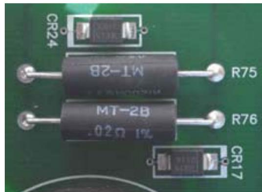
Figure 5. Good hole-fill 0.093 inch thick board.
