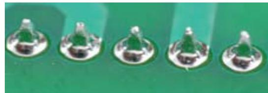
Figure 3. Button-side, bright joints with SnCu based solder K100LD
