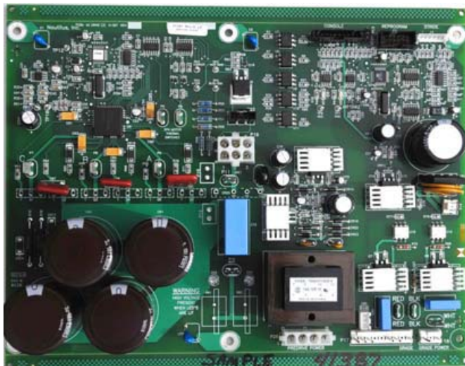
Figure 10. Sn100CL HASL 0.093 inch thick board soldered using K100LD.
