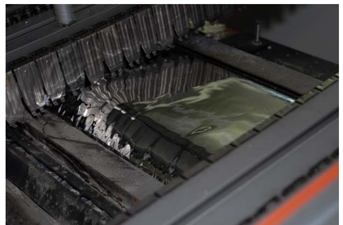
Figure 13. Low dross formed with SnCu based solder
