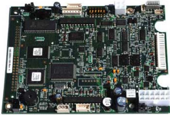
Figure 9. ENIG board with lead-free parts soldered
