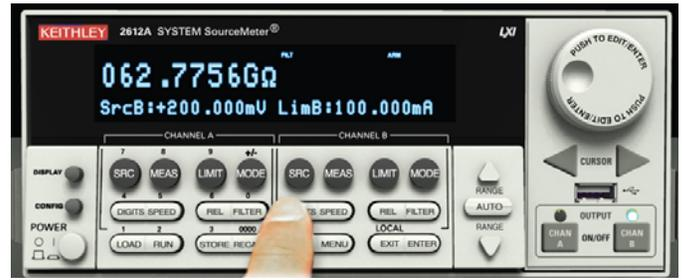
Figure 5. Adjusting an SMU instrument's resolution.
