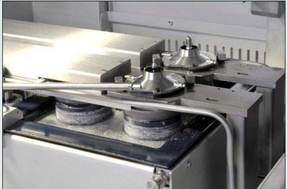
Figure 3: Dual solder fountains on X-Y axes; 1.8mm (left) and 4mm (right). Photo courtesy of JUKI.
