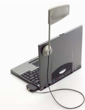
AnalyzeAir software interprets the RF energy in the spectrum or channel and lists the devices that are transmitting – associating real devices with the energy pulses. It automatically identifies Bluetooth® devices, cordless phones, microwave ovens, analog video cameras, and RF jammers. Then the "Device
