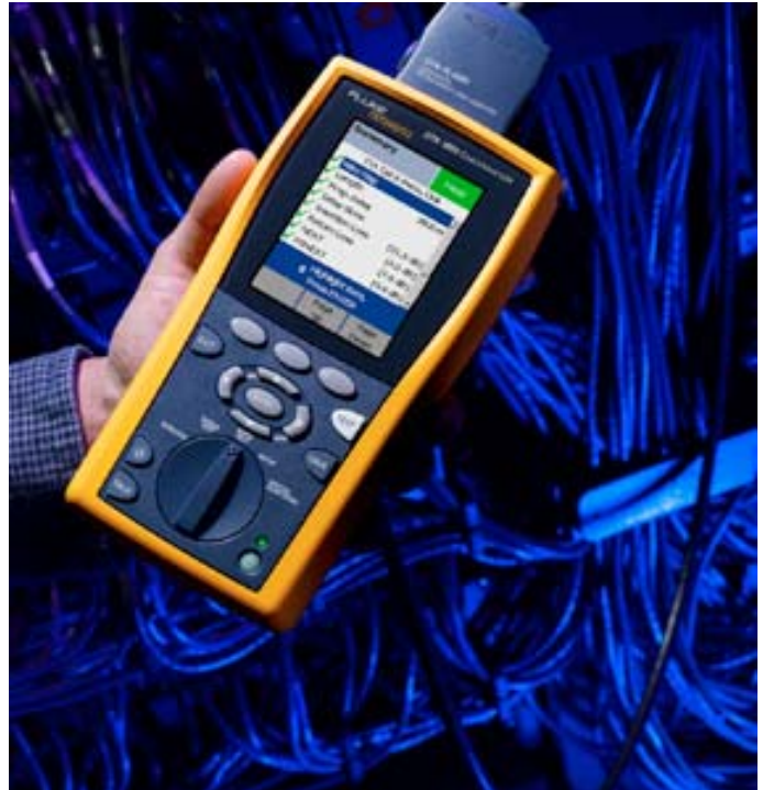
Figure 1. Certification tools take very precise measurements on parameters spelled out in TIA and ISO standards. Documented results from a high-accuracy certification tool is often the only means of meeting the requirements of manufacturers' warranties.
