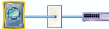
LinkRunner tests for the existence of link - a signal successfully sent and received over a single wire segment.
