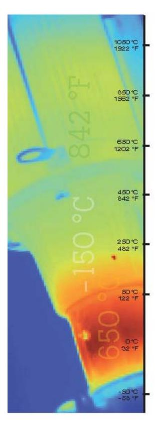
Most painted objects have a high emissivity of about 0.90 to 0.98. Ceramic, rubber, and most electrical tape and conductor insulation have relatively high emissivities as well.
