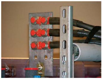
Simple painted markings like theses are often used for highemissivity "targets" that dramatically increase the reliability of radiometric measurements.
