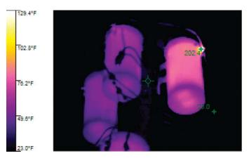
This finding, an internal fault in a pole-mounted transformer feeding a critical load, was considered serious enough that it could not wait for a scheduled shutdown. Protocols should be established before the inspection to handle situations like these effectively.
