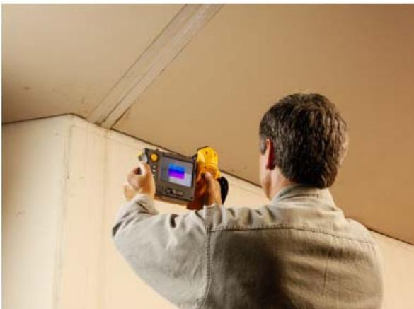
We observe temperature changes from wet to dry as slight at 0.5°F to greater than 10°F. During the drying of a building, the temperature differential between wet and dry will go up or down depending on the ambient temperature of the building and moisture content of the material. For the most part, temperature differentials are greatest the first 24 to 36 hours.
