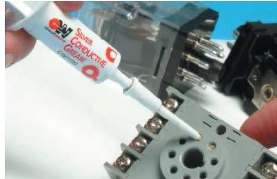
Step 3.2: Apply conductive grease to connectors
