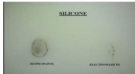
Samples prepared from each of the four soil types tested showed only partial removal of the soil (<50%) after a 5-second spray when using the 99.9% IPA. More than 90% of each soil type was removed by the Electro-Wash® PX
