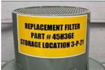
To reduce search time, and ultimately reduce downtime, clearly label **shelves and bins** in stock rooms and tool cribs. Where possible, use graphics and/or photos on your labels for faster recognition and to avoid pulling the wrong part.
