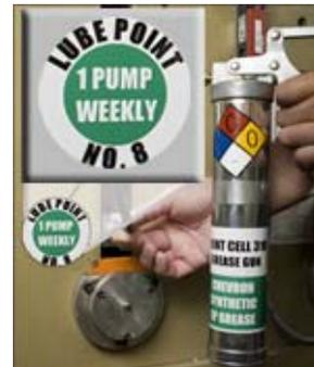
In addition, **color-coded markings** can be applied to zerk fittings and grease guns to guard against using the wrong type of lubrication.
