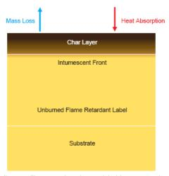
This diagram illustrates how in a polyimide construction heat is absorbed, and the char layer forms a barrier. The oxygen binds when burning and creates the CO2 smoke which becomes the mass loss. This burned off layer protects the underlying material.
