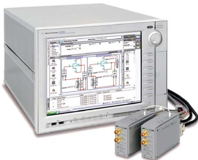
Figure 3. The Agilent B1500A semiconductor analyzer can be accessed remotely to characterize devices
