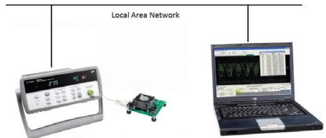
Figure 1. The Agilent 34972A data acquisition instrument takes measurements remotely over LAN
