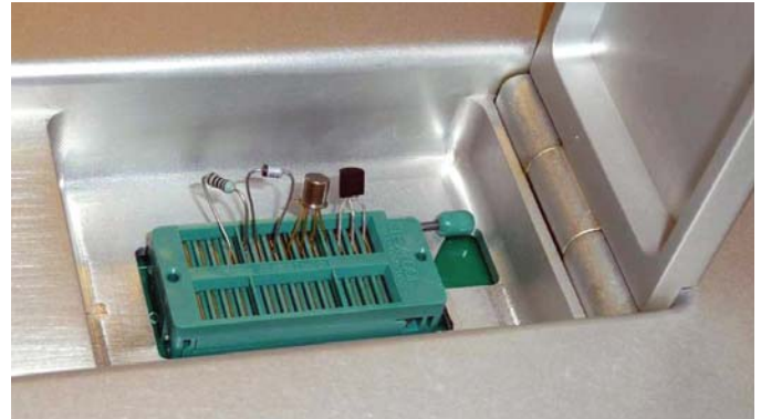
Figure 4. Using a MUX, students can remotely switch between devices under test. From left to right: resistor, diode, mosfet, and bipolar transistor
