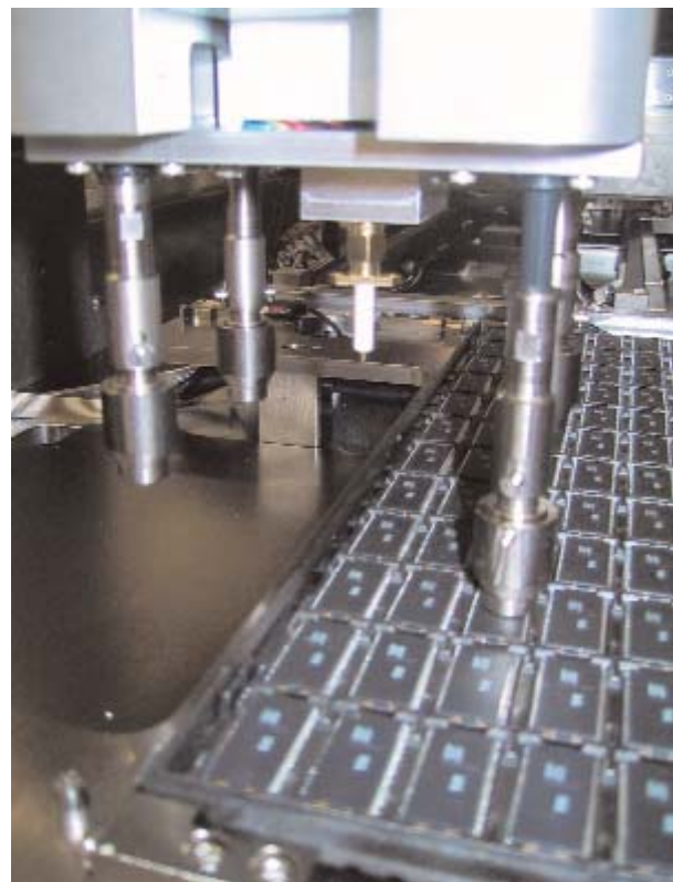
Figure 5: ESD monitor sensor in Epson NS7000 IC handler
